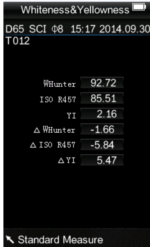
Figure 27 Whiteness&Yellowness Sample Measurement
