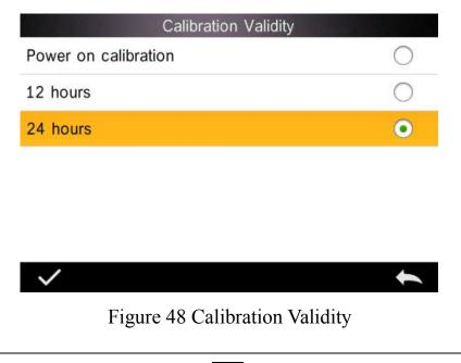
If power on calibration is selected, it could do white and black calibration every time when you turn on the instrument. If not, it would be only able to check records abut not complete the test.
