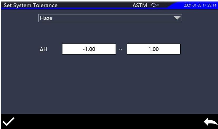
Figure 53 Interface for setting haze tolerance
