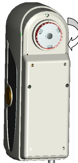
Figure 11 Turn the Measuring Aperture Clockwise About 20 Degrees
