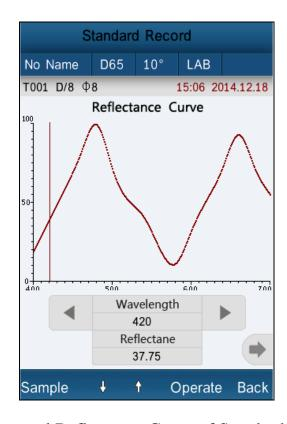
Figure 14 Spectral Reflectance Curve of Standard Record
