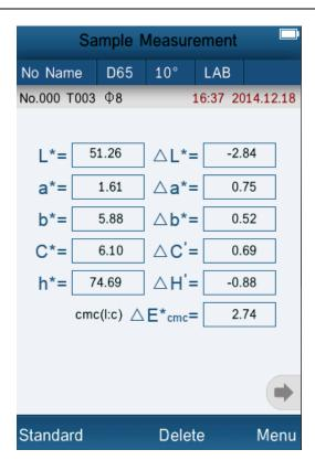
Figure 36 Color Index cmc(l:c) Sample Measurement
