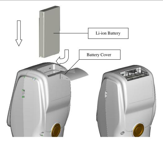
Figure 2 Battery Installation
